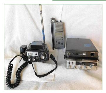
These old radios are still operational after several decades. Left, is a Midland CB from the '70s. The built-in antenna and battery pack have allowed five mike contacts. Center: a 30-year-old scanner. Right, a Mobil CB with SSB, allowing greater range. Normally mounted in a truck, this one's attached to an old Radio Shack Portable Power Pack. This allowed use on the move or at remote locations.
