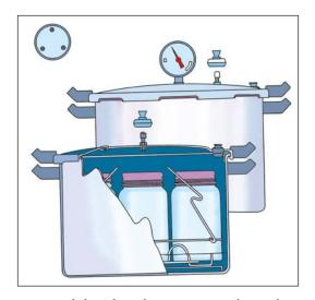
turn-on lids. They have a jar rack, gasket, dial or weighted gauge, an automatic vent or cover lock, a vent port (steam vent) that is closed with a counterweight or weighted gauge, and a safety fuse.
