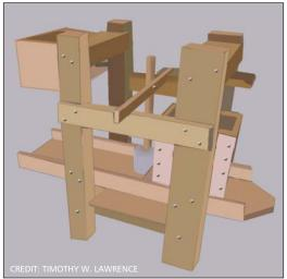
This press works for both making cider and for pressing cheese. The apple press part is a scissors jack (found at an auto parts store) mounted to one of the top timbers. The opposite end is a grinder, made up of two oak rollers. Stainless steel screws serve as teeth to mash the apples, which are then strained in the mesh-lined bucket. You can then press the apples on the opposite end.
