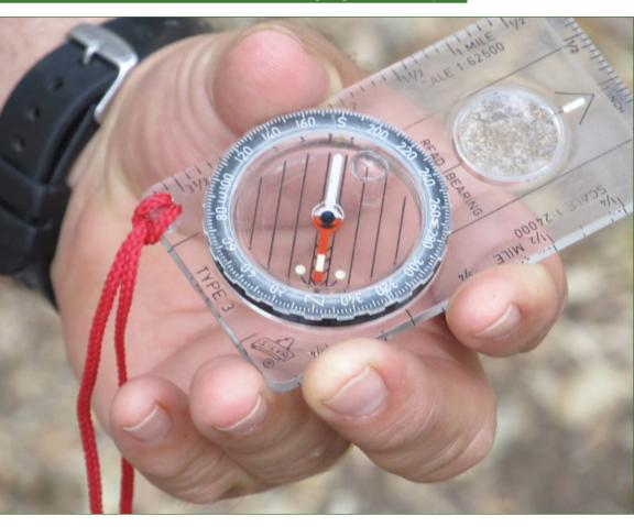
The dog is in the doghouse. The magnetic needle's north end is within the boundaries of the printed arrow on the movable dial of the compass.
