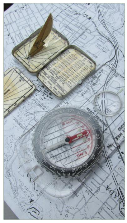
A simple localized sundial that fits into an aspirin tin is actually accurate when made well and adjusted for location.
