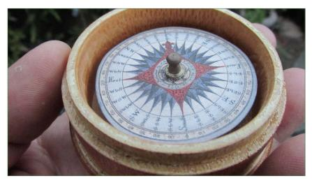
An early style of compass. A magnet secured to the bottom of the round disk, which is balanced on a pin, causes the disk to point to Magnetic North.
