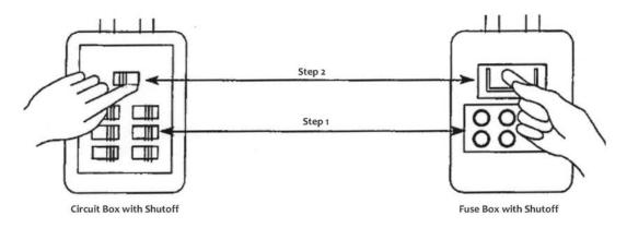
Proper method for turning off the electricity. First shut off individual breakers or pull individual fuses and then shut off the main breaker or pull the main fuse.
