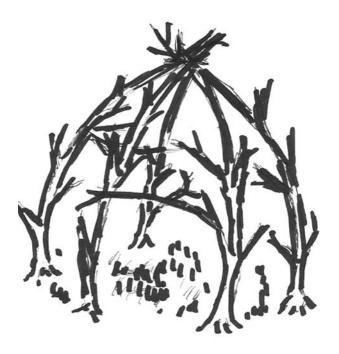
The dome shelter above is strong and can be built with or without an open side, depending on whether you will have a fire or will be conserving heat inside. All you need to do is find bendable saplings. You can cover it with natural or man-made materials. One of these that I built lasted more than two years.
