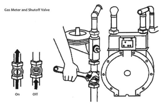
Proper way to turn off the gas supply. Once this is done, you should contact the gas company to have it turn the gas back on safely.
