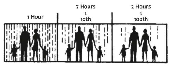
The above illustrates how radiation decays over time by a factor of ten for every sevenfold factor of time. The general recommendation is to remain in as much shelter as possible for as many hours as possible for at least two weeks. This was for a massive nuclear exchange. Limited nuclear strikes or incidents would create less initial radiation and thus shorter shelter times.
