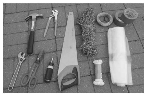
A few home repair tools. Have enough tarps and heavy-duty plastic to cover broken windows and damaged roofing. You should have plenty of rope, wire, tape, and nails as well.
