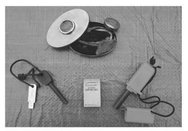
Note also the magnifying glass. Such devices were a must before the invention of the match. Left front is a pocket-sized magnesium spark-striking device. I recommend one of these in every jacket pocket and survival kit. At center is a pack of common camping matches. These are waterproof, but I keep them in a plastic bag anyway. The larger magnesium striker on the right provides a big reliable spark, a must for the full-sized backpack or bug-out bag.
