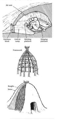
Top: Building this snow cave shelter would be much better than remaining exposed outside. Note the cold air sump and sleeping shelf. Cold air sinks, so a shelf a few feet above the floor could be five to ten degrees warmer. Center and bottom: Bent
