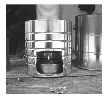
While the homemade hobo stove shown here uses alcohol, it can use twigs or candles as well.
