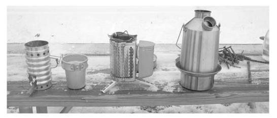
Various versions of the rocket stove use twigs and small branches in metal stoves to maximize the heat from a little fuel. Using the fuel to heat food and beverages that go into the body is much more efficient than using a campfire, which radiates most of its heat into the air. Shown here (left to right) are a surplus Swiss Army rocket stove, a high-tech stove that generates electricity and has its own fan, and a kettle stove that heats water quickly.
