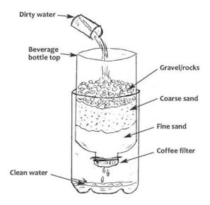
This filter uses a large plastic beverage bottle with the top cut off and inverted. The top layer is clean gravel, followed by coarse sand and then fine sand held in place by a coffee filter.
