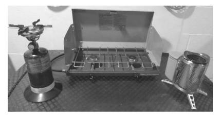
Left and center: A single-burner and twin-burner camp stove. Right: One of the new High-Tec rocket stoves. This one uses a battery-powered fan to blow air through burning twigs so effectively that you can heat a pot of water with just one or two handfuls. The heat also recharges the fan battery and can recharge a cell phone. It's still too dangerous and smoky for indoor use, but the fuel supply is nearly inexhaustible.
