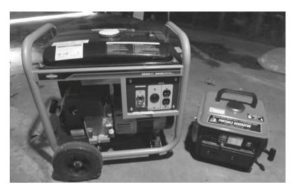
The 100-watt generator on the right is easy to move and uses little fuel. I ran my sump pump and small freezer alternately on this for two and a half days on a few gallons of gas, but, of course, I had to rely on solar lamps and candles for lights. The larger 3,500-watt generator can power most home appliances but burns a lot of fuel in the process.
