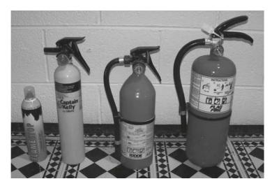
The two smaller, disposable extinguishers on the left may be okay for the vehicle or kitchen, but larger, refillable ten- and twenty-pound extinguishers are recommended for the garage, basement, and central closet.
