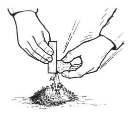
Grasp the flint (or substitute) and steel as shown above. Then strike the edge of the flint. Practice directing the sparks into the starting tinder.
