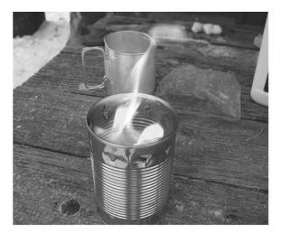
This sand stove is made by filling a can threequarters full of sand and adding enough gasoline (or other flammable liquid) to soak but not cover the sand. This is a good way to use any available flammable liquid safely and efficiently.
