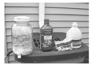
Homemade filter using alternating layers of sand and activated charcoal separated by coffee filters. After filtration, use bleach for biological decontamination of rainwater from the roof.
