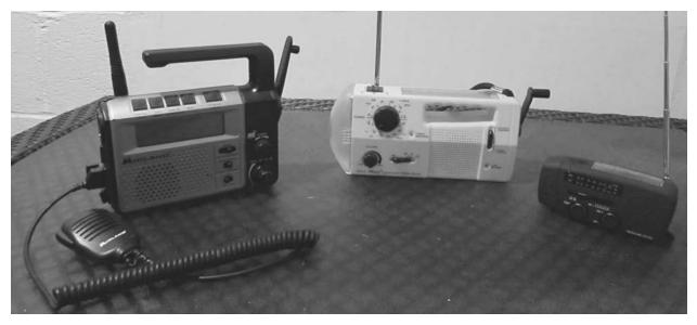
Emergency radios come in many forms. The one on the left is crank and battery powered, and has the capacity to transmit on the GMRS/FRS wavelengths. The center one has a light and a siren, and is crank and solar powered. The small radio on the right has a crank and solar power system, and can even be used to recharge your cell phone.
