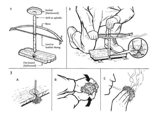
handhold should be made of harder wood. A pine knot works very well. Cut a depression on the handhold to keep the end of the spindle in place. If available, put tallow or other lubricant in the notch to reduce the friction at that end. The bow should be approximately twenty-four inches long and made from stiff, springy wood, such as ash. Notch the ends slightly to keep the string in place. Use a shoelace or other type of cord for the bowstring. A leather thong is best.
