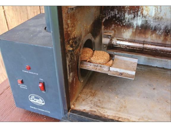
**ABOVE:** The smoke generator feeds bisquettes at a precise burn time of 20 minutes per bisquette.
