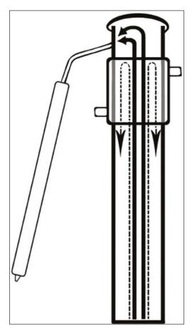
formation to increase the amount of vapor actually affected by the lines. They later increased the number of cooling lines in this formation to further improve efficiency. The result is that a very high portion of the rising vapor will either contact a cooling line or be affected by the cool temperature radiating from them. When this type of column is run properly, and the vapor does finally get past the cooling lines, it is usually of very high purity.
