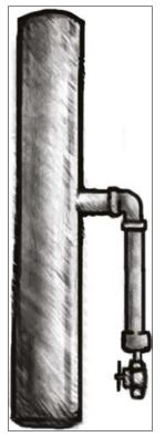
slight modification, that being that you must create the reservoir for the condensate to collect, you can essentially just move the reflux head of an external reflux still to the top of the column to create the internal valved reflux still. Because the design is fundamentally the same, it has the same benefits and drawbacks of the external valved reflux column.
