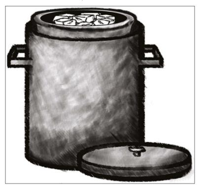
To build the stock pot still, you will need a large stock pot (at least a five-gallon (19L) preferred), a stainless-steel mixing bowl large enough to sit on top of the stock pot, and a slightly smaller stainless-steel mixing bowl that can fit inside of the stock pot with at least 1/4 to 1/2 inch of space all the way around it.
