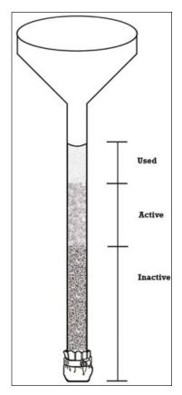
slowly. A good filtration speed using a 105in<sup>3</sup> carbon filter is 1 quart (946ml) per hour, although up to 2 quarts (1.89L) per hour is generally very effective.
