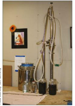
collection container. On forced reflux columns that employ a system such as the internal cooling tubes below the condenser connection, you can eliminate the need for a second step by installing the gin basket between the cooling lines and the condenser. In this design, the highly purified vapor is forced to flow through the material in the gin basket, picking up flavor and aroma compounds on its way to the condenser.
