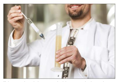
Hydrometers and test cylinders are essential tools for testing samples of your wash.
