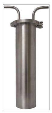
to adjust the fill level. Assuming that the volume of your thumper is optimal for your distillation, a taller and more slender design is much more effective, as it gives the incoming vapor much more contact time with the cool liquid, allowing it the time needed to be condensed and exchange heat with the liquid in the thumper. If your thumper is too shallow, then the vapor may not get condensed, and it will not be effective.
