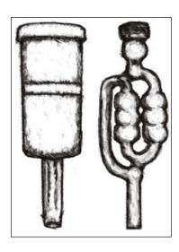
Airlock: An airlock, or vapor lock, is an inexpensive type of one-way valve that uses water to act as the control. There are several airlock designs, but all perform the same job, which is to allow gases formed during fermentation to escape while blocking outside air, which contains oxygen and spoilage organisms.
