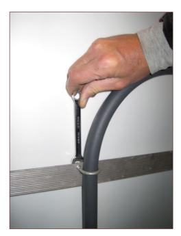
Tightening nut on U-bolt securing panel to hand truck frame. Background is white plastic rear of photovoltaic panel.
