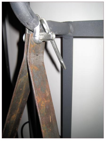
Circular clamp fastens strap-iron stand to hand truck handle.
