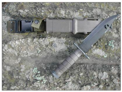
LanCay made the M9 bayonet for the U.S. Army. Oval hole in blade fits over stud on sheath to form a heavy-duty scissor for wire fences and the like.
