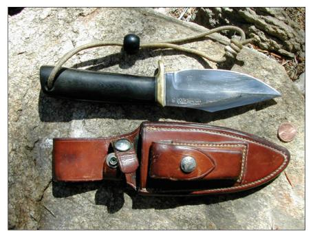
Randall Made Knives<sup>®</sup> model 19 Bushmaster purchased in 1967. Note smooth, Micarta handle and brass guard. Author drilled hole in handle for a lanyard with cord lock. Sheath features a compartment containing a honing stone.
