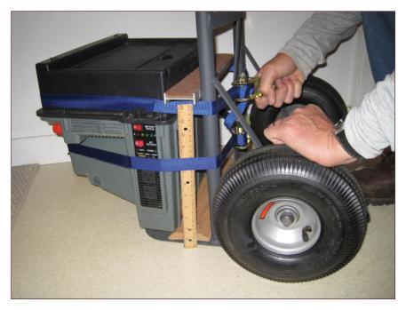
*Tightening blue nylon ratchet straps securing generator case to hand truck frame. Note padded aluminum base for photovoltaic panel. Ruler shows scale.*
