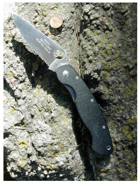
Spyderco military model features blade of CPM (crucible particle metallurgy) 440V, a tough stainless steel. The black scales are G-10.
