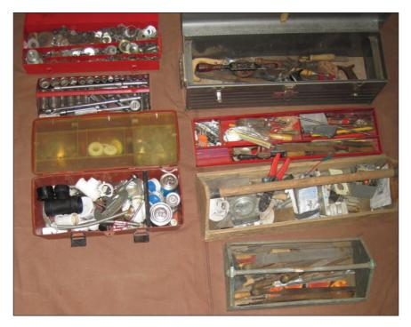
Left: Red metal box contains assortment of washers; red tray holds socket set; plastic box contains plumbing tools, adhesive and supplies. Right: Grey metal toolbox and red tray contain carpentry hand tools; wooden tray holds electrical parts and tools; metal tray is full of files.
