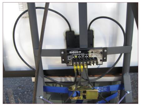
SunSaver-10 charge controller attached to bottom crosspiece of hand truck. Note yellow, weatherproof, heat-shrink tubing on terminals. Background: loops of black wire from rear of PV panel. Illuminated green LED indicates charging.
