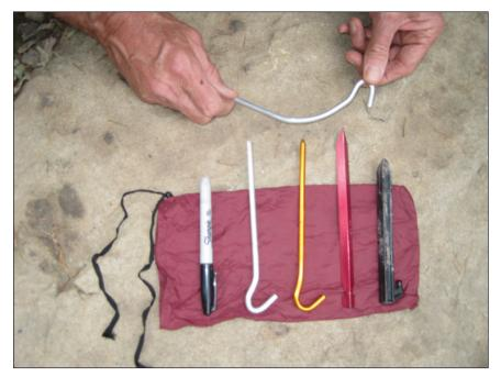
Tent pegs come in a variety of shapes and materials. The bent peg was made from inexpensive aluminum. Marker shows scale.
