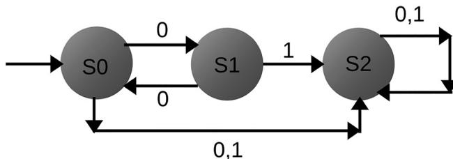
**FIGURE 7.1:** An example of an NFA. Image adapted from <https://math.stackexchange.com/questions/1240601/what-is-the-easiest-way-to-determine-the-accepted-language-of-a-deterministic-fi?rq=1>.
