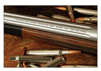
For example, a whitetail deer is similar to a man in size. The .30–06 Springfield is one of the most popular cartridges used to hunt them. With a 150-grain bullet at 2,910 ft/s, it produces 2,801 foot-pounds of energy. A 9mm 124-grain bullet at 1,150 ft/s has 364 foot-pounds of energy. So in effect we are shooting a deer with a bullet carrying 670 percent more energy than that popular self-defense cartridge carries to stop a bad guy the same size as the deer.
