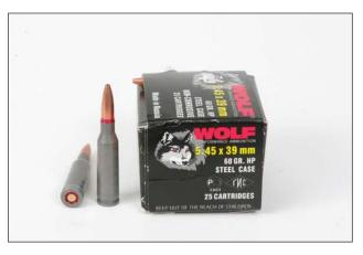
This was Russia's answer to the 5.56 NATO and was developed in 1974 for use with the new AK-74 rifle. Hornady, Wolf, and TulAmmo all offer newly manufactured expanding bullet ammo. Wolf and TulAmmo have 60-grain HP bullets with a MV of 2,960 ft/s. Hornady loads a 60-grain V-Max at 2,810. All of these loads use a Berdan primed, non-reloadable steel case.
