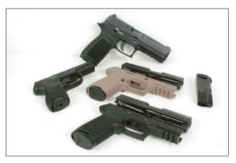
▲ The Sig Sauer P320 handgun is pretty much a "kit" gun. The serial number is on the trigger group, which is removable and portable. So you can switch frames, slides, barrels, and grips to configure the pistol any way you want.
