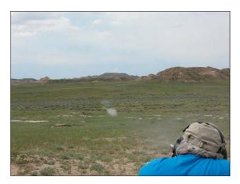
▲ The puff of gray downrange is a bullet disintegrating in flight. This is due to hoop forces generated by too fast a spin rate for the bullet and velocity.
