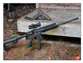
▲ The TRESNA JAG9G BU Tactical Rifle is a 9mm-chambered AR-15 type rifle. It uses the Glock magazines so you can interchange with a Glock 9mm handgun.
