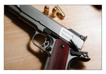
▲ The proper condition for a 1911 is cocked and locked.
