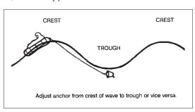
**Figure 16-6** Deployment of the sea anchor.
