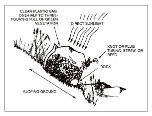
Figure 6-6 Aboveground solar water still.
