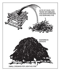
Figure 19-2 Smoke generator—ground.
