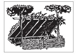
**Figure 5-5** Field-expedient lean-to and fire reflector.
