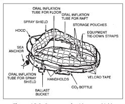
**Figure 16-8** One-man raft with spray shield.
