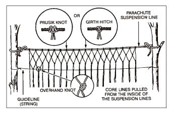
Figure 8-19 Making a gill net.
