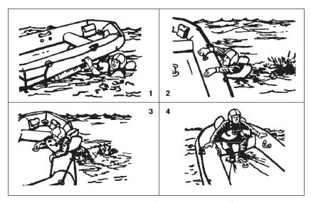
Figure 16-14 Method of boarding seven-man raft.
