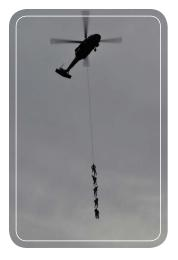
Special Operations Forces (SOF) use S.P.I.E.S (Special Patrol Insertion Extraction System) to rapidly insert and or extract small recon patrols and sniper teams from areas where a helicopter can't land.
