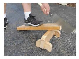
For ripping, use one horse to angle the board up. Start the cut with your crosscut teeth and a thumb to steady the saw but stand up for the long rip-cut.
