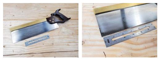
A small, fine saw cuts a narrow kerf and leaves a smooth surface. This saw has 13 teeth per inch. It's great for detail work, but it's too slow to use for cutting up big boards.
