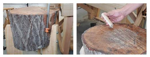
After adjusting your hole, you clamp should slide in and stay in place with friction. Once it's done, drill a hole (or two) in the top of your log to accept a peg. The clamp will hold work down and the peg will keep it from rotating.
