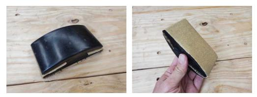
This commercial rubber sanding block grips the paper securely and makes it easy to sand large surfaces with the paper held flat.
