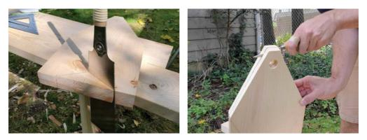
With your two ends stuck together, it's easy to cut the details onto both pieces at once. When you're done, use the knife and the hatchet to slowly force the pieces apart.
