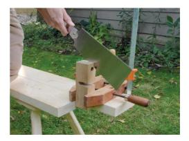
The phone notch is on the end of the organizer. Drill a hole and rip down from the end. You're done.
