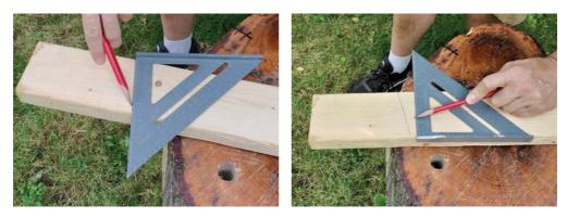
You can use your speed square to easily lay out an angled line. Cut along this line and you have a 15° angle guide.
