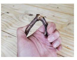
This dead twig splinters instead of bending. Where it breaks, you can see the fibers that make up the wood.
