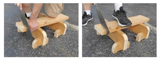
For crosscuts, you can kneel on the work and have both hands to start the saw right on the line. Once your cut is established, stand with one foot on the work and use two hands on the saw.
