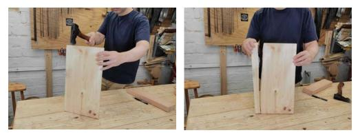
Instead of sawing the edge off this board, I can split it off with a hatchet. Notice that my hand is far away from the split and my fingers are well out of danger. I only use this technique with a wide board so that I can hold it safely.
