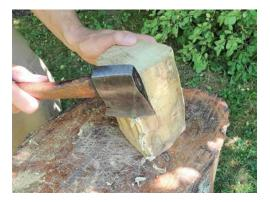
I'm not going to leave any sharp edges on my mallet head. I'll use the hatchet to trim the edges and then a sanding stick around the faces. The final tool needs to be comfortable and resist splintering.
