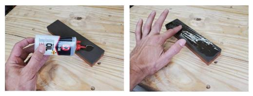
Your sharpening stone should be evenly coated with oil. As you use the stone, little particles of metal will come off your tool. The oil will keep these particles out of the stone. Be sure to wipe off the used oil every time you use it.
