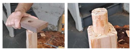
Drill a hole in a scrap of hardwood and use it to test your tenon. At first, the tenon won't fit at all. Trim a little with your knife and try again. Once your test board slides on a little bit, you'll be able to see crushed, shiny fibers and a little ridge where the test-board stopped. These signs will tell you where to trim.
