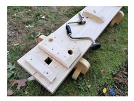
Before I glue in the legs, I'm screwing on the small battens. These are made from the extra legs I didn't use. I put one batten in the middle of the bench and one at either end. The exact locations don't matter.
