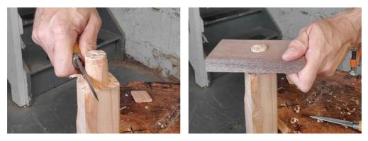
Trim carefully with your knife, taking very thin shavings. At this stage, little changes make a big difference. After several rounds of trimming and fitting, your test-board should slide all the way to the shoulder.
