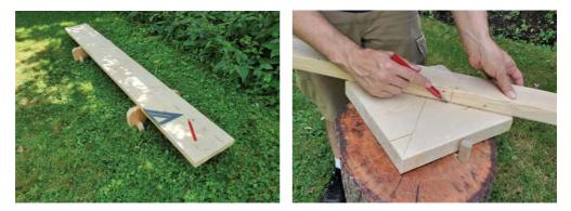
My seat comes from this SPF  $2 \times 12$ , but any solid wood will do the job. Your low sawhorses can easily support this big board for crosscutting. Use a straight scrap of wood to connect the corners of the square and you'll have the center.
