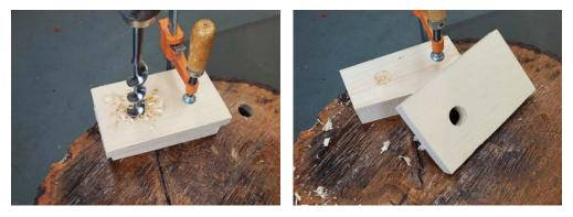
*I* drilled this hole from both sides, but *I* also clamped a piece of scrap underneath during drilling. The scrap supports the fibers to minimize damage if you break through by accident.
