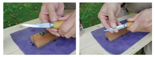
On the left, you can see that the first  $\frac{1}{3}$  of the blade is covered in fine scratches all the way to the edge. On the right, I'm pushing my fingertips across the edge from the underside. As my skin moves over the edge, I should feel the burr.
