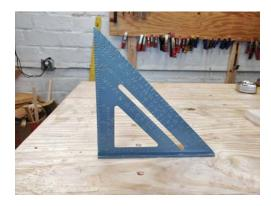
A basic speed square is a cheap and useful measuring device for the shop.
