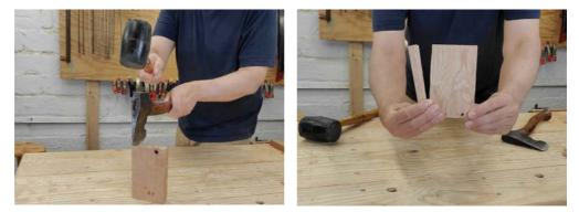
By placing the edge of my hatchet exactly where I want to split the wood and then striking it with a rubber mallet, I get to choose exactly where the wood splits. This technique is safe to use, even on small pieces of wood.
