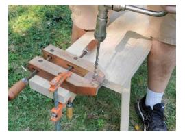
Your two clamps can work together to hold small pieces for drilling and carving.
