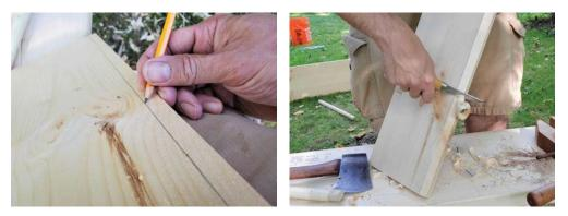
You can lay out your bevel by letting the nail and knuckle of your middle finger ride against the edge while you hold your pencil at the distance you want. This simple technique is surprisingly accurate. After most of your waste is chopped away, finish up with a planing cut from the carving knife.
