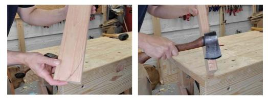
Trace a curve across the corner of a piece of wood and then remove everything outside the curve. Start with a series of light chops to weaken the fibers.
