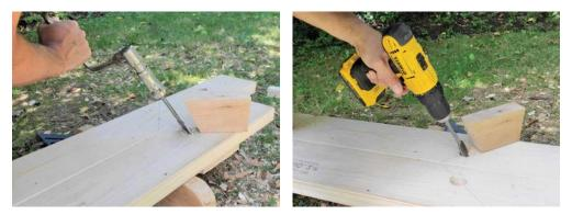
Whether you drill with the brace or an electric drill, line your bit up with our 45° lines and then bring in the angle-block.
