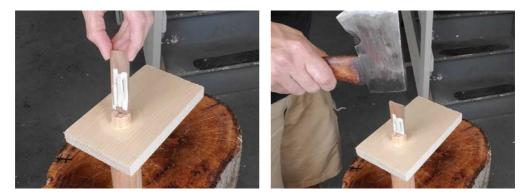
I put glue around my tenon before inserting it in the mortise. Now, I've got glue on my wedge and I'm inserting it into the slit and tapping it home with the back of my hatchet.
