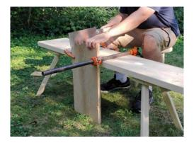
You can hold wide boards against the edge of your bench by adding one more long clamp. In the picture, I've clamped my work to the far side of the bench so that my pull-saw can work effectively.
