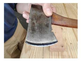
If you can't tell where you've sharpened your tool, try coloring the bevel with a marker. In this picture, the marker has been rubbed away where I sharpened the very edge. That's good, but I also want to work the bevel. I'll return to the stone and take several more strokes, adjusting the angle of the tool until all the marker is rubbed away.
