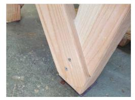
I used screws and construction adhesive for this joint in my workbench. Screws work well for shop furniture like benches, especially with a good design that won't let them loosen over time.
