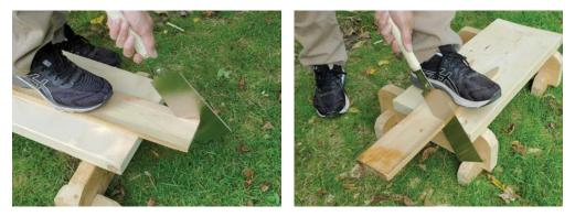
Use the rip teeth on your Ryoba to cut out the V-notch. Stand on your work to hold it steady. This is where using a long piece of stock comes in handy. After the notch is done, crosscut to final length.
