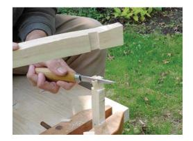
small pieces. If I'm carving a small tenon (a little joint) on a delicate piece of stock, I'll saw my shoulders and then baton off the waste with my knife and a scrap of wood as the mallet. Remember to take small cuts and strike the spine of your knife gently.
