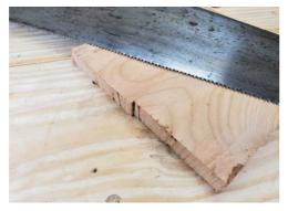
When you saw a piece of wood, you turn some of it into sawdust. I sawed this board in half, but the lefthand piece is a little bit longer because of the kerf.
