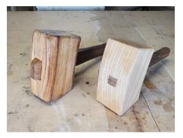
Both of these traditional mallets have handles that extend all the way through the head. While this construction is very sturdy, it's also difficult to make.
