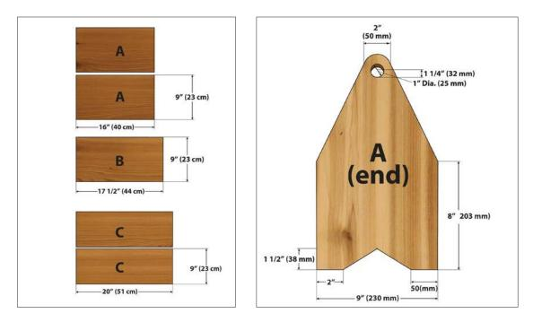
Most of this project is cutting and shaping the ends (**A**), since they have most of the details. To end up with two identical pieces, it's helpful to fix them together and work on both at the same time. Stick a few pieces of masking tape or blue painter's tape to your ends, dab on a little superglue and press the ends together for 30 seconds. The glue will fix your pieces tightly together, but the tape will make it easy to get them apart without damaging the wood.
