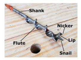
The parts of an auger bit. Some drill bits have fewer parts, but they all work in a similar way. Understand this bit and you'll understand all of them.
