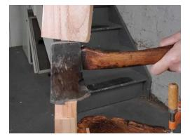
You can use your hatchet to split most of the waste off your tenon. A piece of  $2 \times 4$  makes a good mallet. Notice how the stop-cuts keep the splits from traveling too far down the leg.
