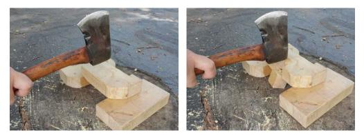
One hard strike with the back of the hatchet should knock out your waste with no trouble, although you may need to use the knife to square up the bottom of the notch.
