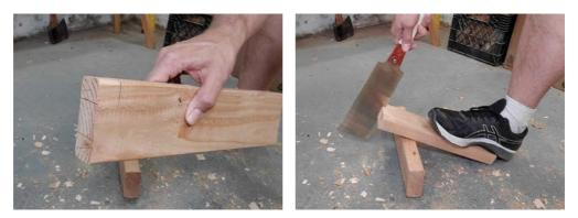
I only sawed the lines I could see, so now I need to flip this board over and finish the rip from the other side. Once I rip down the other side, there will still be a little "triangle" of wood at the base of the cut. I lift my arms so the saw is perpendicular to the wood and finish the cut square.
