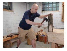
When using the hatchet to shape larger pieces of wood, be sure to stand with your right leg back (if right-handed) and out of the way.
