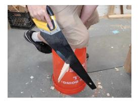
A plastic bucket can make a good platform for sawing. Use the weight of your body to keep the wood steady as you saw it free.
