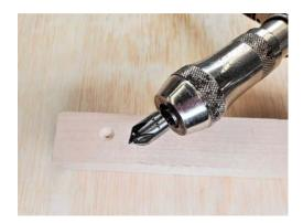
The countersink is a simple tool that works in a drill or a brace. Cut your countersink before you drill your holes and you're guaranteed to get a smoother result.
