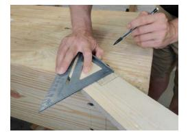
Your square's built-in ruler makes it easy to mark distances on a board. Here, I've used the ruler to mark out a 2" (52 mm) notch that I'll cut out for a project.
