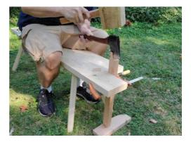
The little corner on the end of your bench makes a great place to clamp narrow stock. In this picture, I put a scrap under my stock to keep it from sinking into the ground as I hit it.
