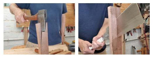
*I'd like to split this piece of wood in half, but the grain is not cooperating, and my split is crooked. If I rip the same piece of wood with the sau, my cuts stay straight no matter what the grain does.*
