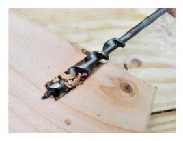
If we look inside the wood, we can see the auger bit working. The snail pierces the wood and guides the bit. The lips break up the wood. The flutes carry the chips out of the hole.
