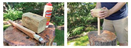
Before I assemble the mallet, I coat all the surfaces with glue and insert my wedge. Then I put the handle in the head, make sure it's turned the right way, and start taping it against my block. As I drive the handle in, it tightens.
