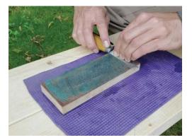
Place your blade with the bevel flat on the strop and pull it toward you with firm downward pressure. Repeat. In the picture, you can see the middle of my strop getting dark as it rubs steel off the knife.
