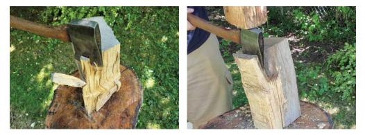
To trim the stock for the head, I'm putting the edge of my hatchet where I want a split and hitting the back with another piece of firewood. This approach gives me both control and power, and the log is quickly trimmed.
