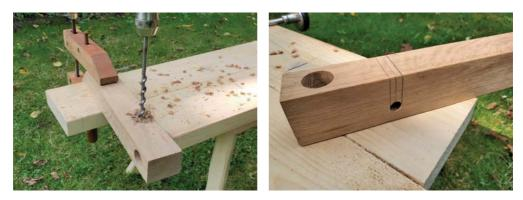
To make a slot, start by drilling a hole. Then use your square to strike lines from the edges of the hole and carry them around the side and onto the opposite face.
