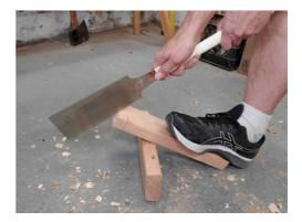
Using a scrap of wood as a sawhorse lets me stand on the wood and still see it clearly. I start my cut with the fine crosscut teeth, and then switch to the big rip teeth and a powerful, two-handed grip. With this stance, ripping is easier.
