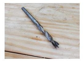
Brad point bits are designed for wood. Like an auger, they have a sharp point and nickers that slice the wood.
