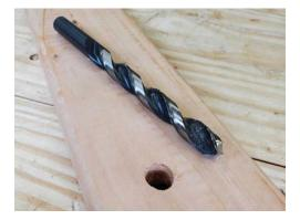
Twist bits are simple, cheap and effective, but they're not designed for wood. Larger bits might tear the fibers a little. Notice the ragged edges on this hole.
