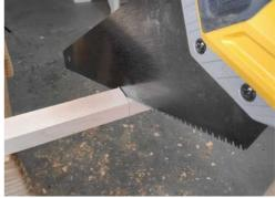
*I've drawn two lines on this piece of wood to guide my sawing. As I cut, I'm careful to stay in the waste side, to the right of my line.*
