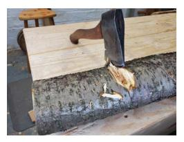
I chopped into this log for over a minute and I've barely dented it. Axes are bad at cutting across the grain.
