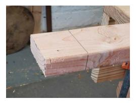
A clear cutting line goes over the face and down the edge of your board.  $2 \times 4$  stock is sold with the corners rounded off, so your line might not meet in the corner.
