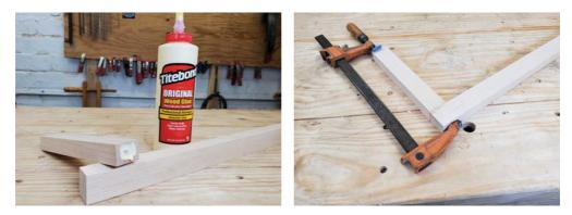
These two pieces can be connected with a "butt joint." A little glue and clamping pressure will make them stick together.
