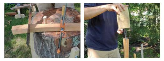
My chopping block is a good surface for small cuts like sawing away extra length. My handle is also too thick, so I split it to width using my mallet head to drive the hatchet. Even without a handle, my mallet is already useful.
