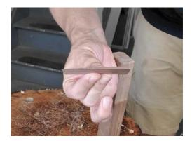
I sawed this wedge from a scrap of walnut. It tapers to a featheredge and is much longer than I need. I'll be able to drive this wedge deeply into the joint.
