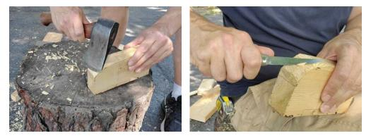
The corners can be quickly shaped with the hatchet and knife. When I use the hatchet, the hand holding the work is far away from the cut. When I refine the curve with the knife, I work off the side of my lap where a slip of the blade can't cut me.
