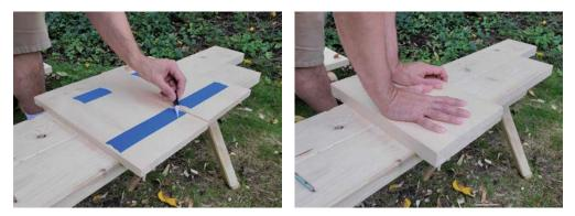
Put pieces of tape on both your ends and add a line of superglue on the tape. When you press the ends together, the glue will stick the boards together, but because it's only on the tape, you'll be able to separate the parts later.
