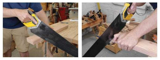
*Left:* Grip your saw with your index finger pointed. This hand position will help you cut a straight line. Right: Press the knuckle of your left hand against the blade of the saw to keep you on track as you begin your cut.
