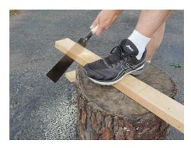
Once I've started my cut, I hold the wood with one foot and grip the saw with two hands for long, powerful strokes. Notice how I'm sawing both the face and edge of the board at once. With my saw following both lines, I'm much more likely to get a square edge.
