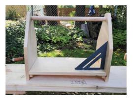
With the dowel in its holes and the bottom resting on the cleats, I can use my speed square to make sure the ends are square to the bottom.
