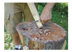
After you've tapered the sides, rotate the leg and trim off the corners. Clean up the cuts with a sanding stick and you'll end up with a nice octagon. Down at the foot, the taper can be as narrow as 1" (25 mm). A narrow foot makes your stool look light.
