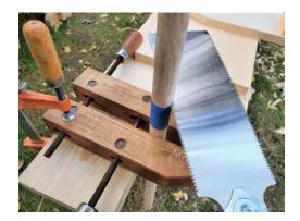
A piece of tape wrapped around a dowel makes it easy to get a square cut. Just follow the edge of the tape.
