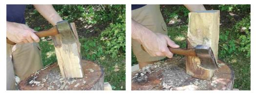
To trim off the ugly surface of my log, I'm gently chopping down half of one side and then flipping the log over and chopping off the rest. Note that my other hand is holding the log by the top of the far side and my fingers are never close to the cut.
