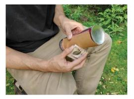
Sandpaper wrapped around a spray can will add a scallop detail to the edge of this piece.
