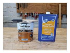
Oil-based polyurethane can be used straight from the can, but I thin it with mineral spirits.
