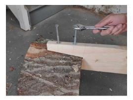
Run your screws in with an adjustable wrench (or a socket wrench if you have one). Get them good and tight. If you try to tighten them later, the screws are likely to snap.
