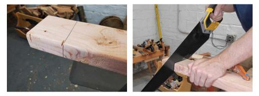
Pulling back several times with the saw will make a little groove that will guide the cut. As you saw through the board, concentrate on pushing gently forward and keeping your saw straight up and down.
