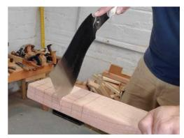
If your blade bends on the push stroke, you're probably sawing too hard or twisting the handle. Try to relax and keep the blade straight up and down.
