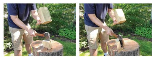
A hatchet plus a mallet gives you both power and control for splitting. Instead of swinging the hatchet, you can place it anywhere on the work and then tap it with the mallet.
