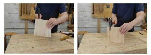
Another safe and accurate way to split wood is to put the edge of your hatchet where you want the split and then keep it in contact with the wood as you lift them both and strike them against your work surface. Don't expect to make the split in a single hit. Make the split with several, controlled strikes.
