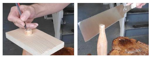
Mark your tenon perpendicular to the grain of your seat-board and then saw down that line.
