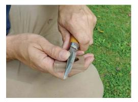
I can easily bevel this edge with a push-cut.
