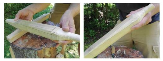
To make tapering the upper leg easier, I've drawn some lines along each corner. Notice that my lines are wider at the top of the leg. I can easily remove the waste with my knife and follow up with a sanding stick.
