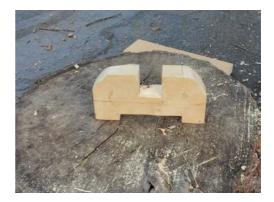
*My* foot is roughed out, but the top notch has a splintery bottom and the walls need to be widened to fit the beam. The knife and sanding stick can handle these tasks.
