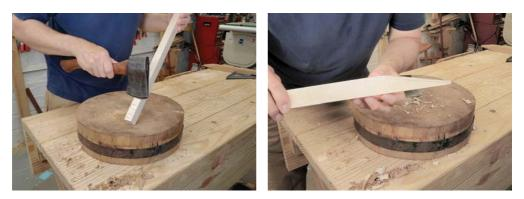
*As I shape my wedge, I'll peel off layers of wood until I'm close to my line, then I can flatten my surface with the hatchet or with a sanding stick.*
