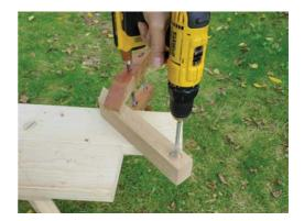
An electric drill and a big spade bit make this hole easy to bore. For this project, I'm using the workbench from Chapter 19, but you can use a board on the low sawhorses, just like we did for the bootjack.
