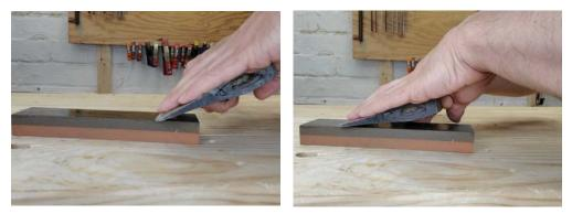
Your basic sharpening stroke starts with the tool up on its edge at about a 25° angle. As you push forward along the stone, slowly rock the tool back so that you transition from the edge to the bevel. At the end of your stroke, the edge is off the stone and you are only working the bevel.
