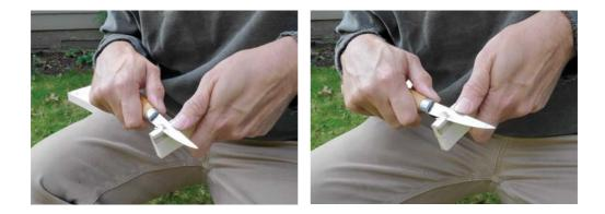
**Thumb Push Cut**: This is a detail cut for removing small amounts of wood. Hold the work in your left hand with your thumb extended. Place the knife against the wood and use your left thumb to push the blade forward. Alternately, you can lock your thumb in place and lever the back of the knife around the tip of your thumb. Both of these cuts offer excellent control and added leverage if you need to cut deeply. I often use this cut when working into a tight curve.
