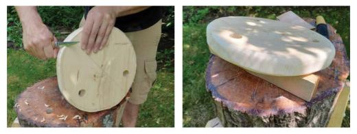
My knife quickly slices a bevel around the edge of my seat. Notice that I've sketched a line about  $\frac{1}{2}$ " (13 mm) inside the rim. I did this line by eye, but it will keep my bevel consistent. After I carve away the waste, I can round the bevel over with the sanding stick and some sandpaper held in my hand.
