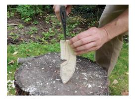
I would never chop this close to my fingers. Instead, I'm lifting the wood and the hatchet together and letting them both fall gently onto the block. One or two taps will split off this big piece of waste.
