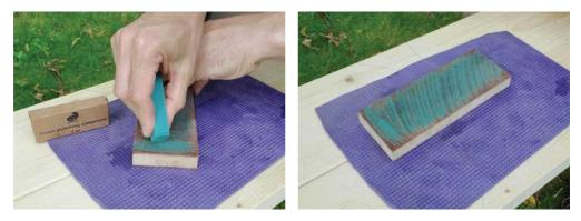
To make my strop, I glued a piece of old leather to a piece of MDF (a cheap particleboard) that's very flat. Then I colored it in with green buffing compound.
