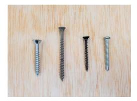
Left to right: wood screw, deck screw, drywall screw, sheet metal screw. Note the "bugle head" on the drywall screw and the round head on the sheet metal screw.
