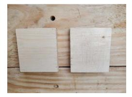
I sanded both of these pieces with coarse, 80-grit sandpaper. Both pieces are deeply scratched, but for the left-hand piece, I sanded with the grain and the scratches blend in. For the right-hand piece I sanded across the grain and the scratches are very obvious.
