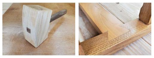
Two joints. On the left mallet with the head and handle joined in **mortise-and-tenon** with a wedge for added holding power. On the right is a simple **dovetail**. The angled sides of this joint help hold it in place, but it still needs a bit of glue.
