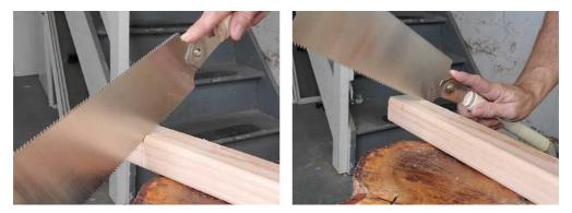
*I've drawn a shoulder line on the end of my leg and now I'm sawing that line all around the leg. This creates a stop-cut like we used in Chapter 5.*
