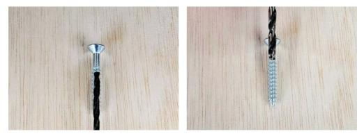
Finding your drill bits is easy. The pilot-hole bit should let the screw threads show on both sides. The clearancehole bit should be slightly larger than the screw-shank.
