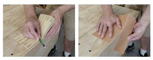
Sandpaper is difficult to cut but it's easy to tear. Fold it over and use a pencil to make a sharp crease, then use the edge of a table to support the fold while you tear. You'll quickly learn how to get a clean and straight line.
