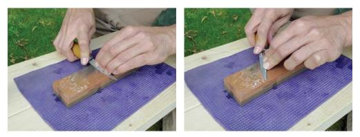
After you've sharpened the first section of blade, move the knife over and sharpen the next section. I can usually sharpen this knife in three sections. As you get near the curved tip, you probably want to skew the blade to put more of the bevel in contact with the stone.
