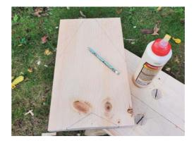
The layout for your ends is just a few lines, and your glue bottle makes a nice radius for the arc at the top. Put a little squiggle of pencil in the waste to remind you what you're cutting away.
