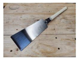
Like the contractor's saw, the Ryoba comes with hardened teeth that stay sharp a long time but cannot be sharpened. When this saw does get dull, you'll be throwing away the blade. Luckily, the blades on Japanese saws are replaceable, so you get to keep the handle. Replacement blades for these saws are reasonably priced.
