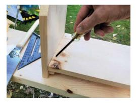
Screwing through the bottom and into the cleats will tighten up the structure. In the picture, you can see a small gap between the bottom and the end. As I tighten my screw, that gap will close.
