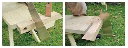
To saw out my notch, I remember the "triangles" rule from Chapter 7. I saw the lines I can see, flip the piece, and saw the lines on the other side. I finish up by bringing the saw perpendicular and sawing the final triangle hidden inside.
