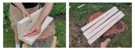
To lay out your legs, use the edge of a board. I ripped piece C into six legs and then picked out the best four. The two legs I'm not using can be cut up to make three small battens.
