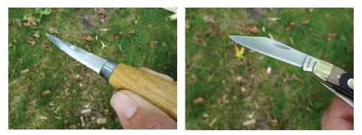
The carving knife on the left has a single, wide bevel that's great for woodworking. The pocketknife on the right has a narrow secondary bevel. It cuts, but it's hard to control.
