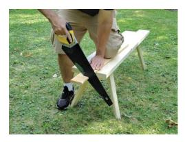
Sawing on your low bench is easy. Your body weight holds the work and you can get right on top of the cut.
