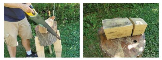
*I* can use my chopping block with the clamp to hold my log while *I* saw it to length. In the finished piece, you can see the slight angle on the end. Both the striking faces should be angled this way.
