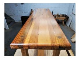
This benchtop is made with many thin boards laminated together. The wide glue surfaces and long-grain connections make these joints strong and durable.
