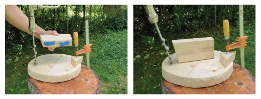
Begin drilling along your sight line with your drill held straight up and down. When the hole is started, add your guide block to give you the correct angle.
