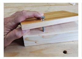
Drop your screw into the clearance hole and then use the point to find the pilot hole. When you use the screw to line up your holes, you save a lot of fumbling around.
