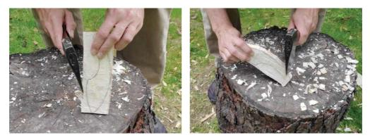
To cut the outside curves, work from the middle to the tip. As you round each curve, keep the hatchet chops straight up and down and slowly rotate the work.
