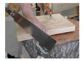
With a clamp and a peg you can hold wood still for sawing or chopping.
