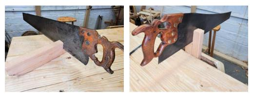
On the left, I'm crosscutting a board to make it shorter. On the right, I'm ripping a board to make it narrower. I'm using a different saw for each cut and these saws are each designed for one kind of cutting.
