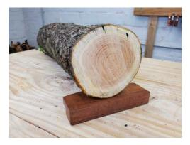
This fresh-cut log is heavy and full of water. Some projects can be made from this "green" wood, but most furniture is made from boards that have been sawn and dried. The log is resting on a small piece of kiln-dried board.
