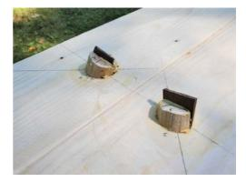
Well-made wedges can be driven firmly and will stop moving before the wedge is buried in the tenon. If your wedges are disappearing into the leg, try cutting thicker wedges with a steeper taper.
