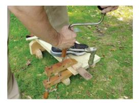
Drilling the hole carefully from both sides gave me clean edges. For now, I'm leaving it attached to the main board.
