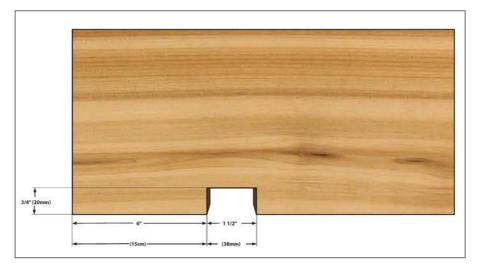
Lay out this pattern on your boards and then carefully saw the lines with your Ryoba. Once you've knocked out the waste and put the boards back together, you'll have a square mortise.
