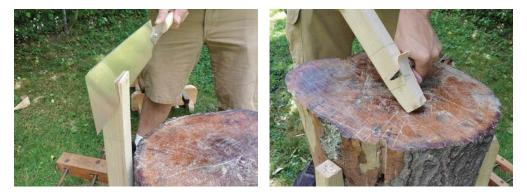
Ripping at a slight angle will start your taper. Follow up with the knife and you can "plane" off the saw marks and get a smooth surface.
