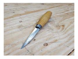
to give you lots of control. The handle is comfortable, and the knife comes with a sheath. You don't have to buy this model. Any small, slightly curved knife with a wide bevel will work. (Many tool makers refer to this bevel style as a "Scandi grind" so that's what to look for.)
