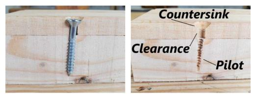
I installed this screw and then cut the wood in half to show what happens inside. Note how the three holes each work differently. The threads bite deeply into the **pilot hole**. The **clearance hole** doesn't even touch the screw shank. The **countersink** cradles the screwhead and allows it to pull against the threads.
