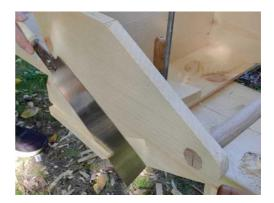
My sides aren't even with my ends, but I left them long on purpose. I can flush-cut the sides, referencing the Ryoba off the end-pieces to get a perfect edge. In this photo, you can also see the handle installed and wedged.
