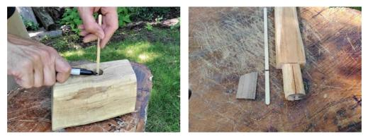
Any stick of wood will make a depth gauge for finding the length of your tenon and your wedge. Both of these must be **less** than the depth of your mortise.
