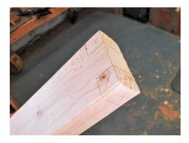
*I've laid out 1" (25 mm) notches on all four corners of this board and drawn Xs to mark the waste.*
