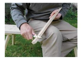
against the spine and skew the blade so the tip points toward you a little. Push forward with a slow, controlled cut, moving the work along the edge toward the point as you cut. Try to take one long, very thin cut all the way along the board edge. If you'd like a wider bevel on your stock, take several light passes, rather than one heavy cut.
