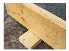
To get my center notch dead on, I mark one side and then lay a piece of  $2 \times 6$  along my line and trace the other side. By marking the exact width of my stock, I'm guaranteed a tight fit when I attach the feet to the beam.
