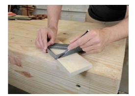
Hold the lip of your square against the side of a board and strike a line across the edge. Your line will be perfectly square to the edge of the board. Saw along the line, and your cut will be square.
