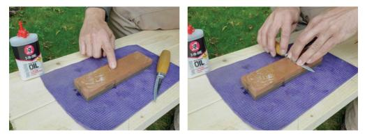
Coat your stone evenly with oil and begin sharpening at the base of the blade. Remember to lay that bevel flat on the stone and keep it there.
