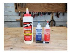
Three common glues. Yellow PVA is sold as wood glue and it's the most common for woodworking. Two-part epoxy comes in two bottles and forms a clear, strong bond. CA glue comes in little tubes. It's great for fast, small jobs.
