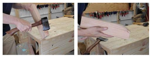
Once you've chopped into the waste, strike down with your hatchet to shear off a layer of wood. Repeat this chopping and shearing until you've removed most of the waste.
