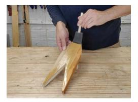
The bootjack will see hard use, so I'm finishing it with oil-based poly. I've thinned the finish with mineral spirits so I can use a foam brush.
