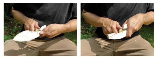
To finish the tight curve, I work into the stop-cut from both directions with a controlled push-cut. Notice that *I'm peeling away thin slices and always keeping my left hand behind the knife.*
