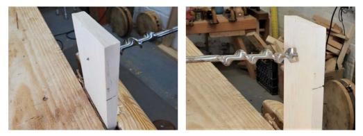
To prevent blowing out the far side of your hole, drill until the point of your bit pokes through, then flip the board around, put the bit into the hole, and finish drilling. The finished hole will be clean on both sides.
