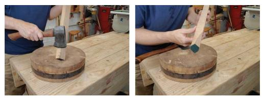
Use the techniques from the last chapter to chop and peel one corner off the stick. Try to leave a flat and even surface. Take off all four corners and you'll be left with a hexagon.
