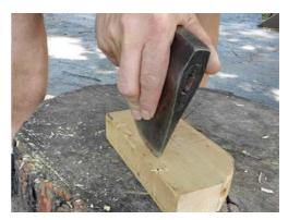
To chop out the long notch at the bottom of the foot, I start by sawing the vertical lines and scoring the horizontal line with the edge of my hatchet. A nice, deep score-line will give me a straight split in the next step.
