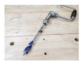
Modern auger bits are somewhat like vintage bits and some work well. (The one in the picture is okay, but not great). To use modern auger bits with a brace, you'll probably want an adapter like the one shown.
