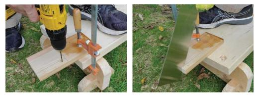
Drill your clearance holes before you saw the cleat free. Large pieces are always easier to hold.
