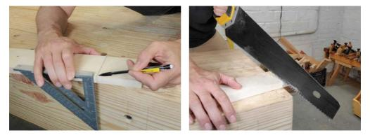
Flip your square so that the lip rests against the face of the board and you can use the edge to strike a line that meets your first line. These two lines meet at a perfect right angle and are very useful for guiding your saw through a cut.
