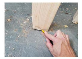
A pencil and a scrap of wood will make a marking tool that scribes the plane of the floor onto your legs. Crosscut this line and your leg will sit steady on the floor.
