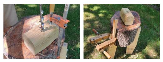
After I drill a hole in the bottom of my mallet, I can clamp the handle-stock to the chopping block and carve the tenon on the end.
