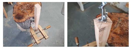
You can screw-clamp the leg to your chopping block and have free access to the end. Once you've found the center of your stock, drill down to score a circle in the end.
