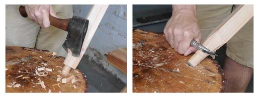
The hatchet and the knife will quickly turn your shoulder into a taper. A little sandpaper helps smooth the transition between the taper and the tenon.
