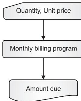
**Figure 1.1a** A System Flowchart Example
