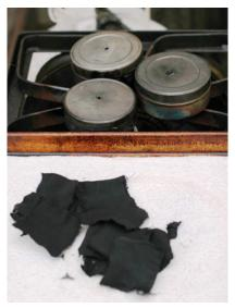
Charcloth is a material that catches sparks. The organic material is "cooked" at a high temperature in an airless container with an exhaust hole, whereby the cloth is changed through a process called pyrolysis. The charred cloth becomes a source of fuel with a very low ignition temperature.
