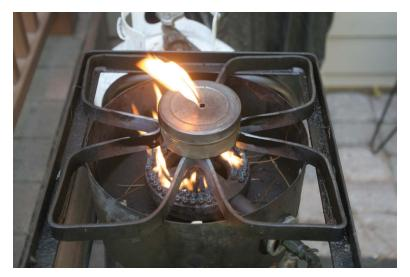
Cook the filled tin outside. The smoke will ignite. When the flame dies down, take the tin off the heat source and let it cool completely.
