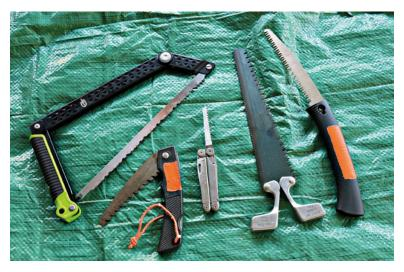
These represent several different styles of saws. (From left) A takedown bow saw, folding limbing saw, Leatherman saw, Pac-Saw, and wood saw with push blade.
