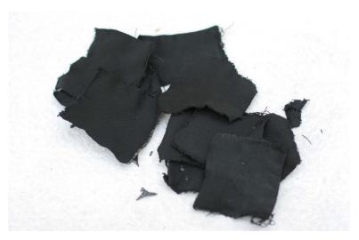
The finished charcloth should be completely black and slightly flexible. When done correctly, the finished charcloth should easily catch a spark and grow into an ember.
