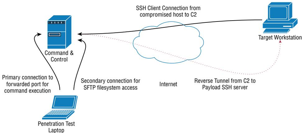
**Figure 1-11:** Initial basic Command and Control infrastructure.
