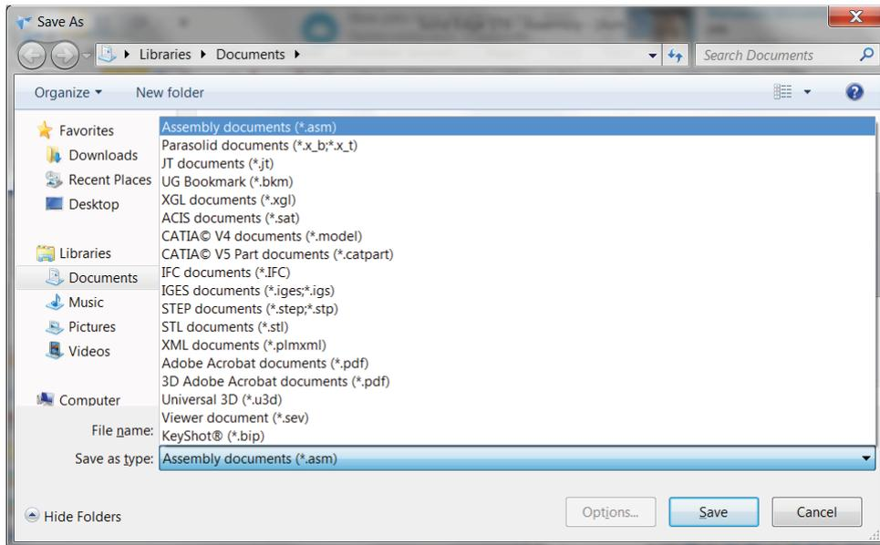
**Figure 5-11:** A Save As dialog box shows the file types Solid Edge works with.
