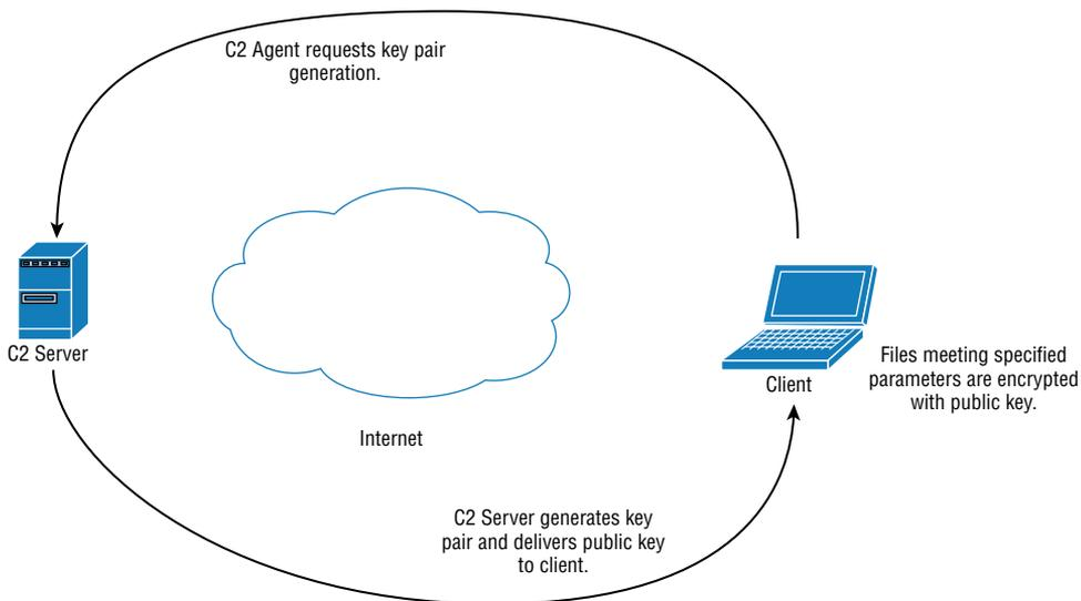
**Figure 5-3:** Encryption process flow.
