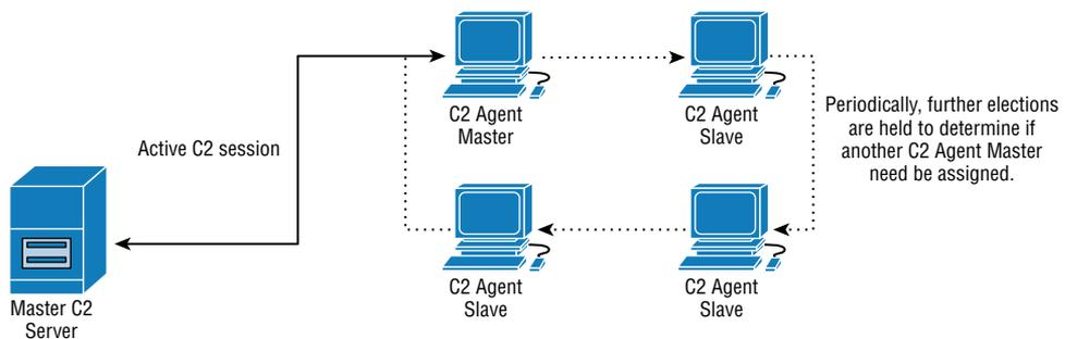
**Figure 8-7:** Further elections are held as necessary.
