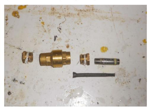
The idea is to create a single acting steam engine (meaning the steam only acts on one side of the piston) by using a pushrod inserted through the spark plug hole to push open the check valve when the piston is at Top Dead Center
