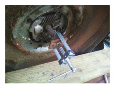
I purchased 5 bolts, 10 washers, 1 lock nut, and 4 1-inch spacers for about \$15 to not only attach the engine to the plate adapter but also to align the pulley on the mower to the one on the alternator.
