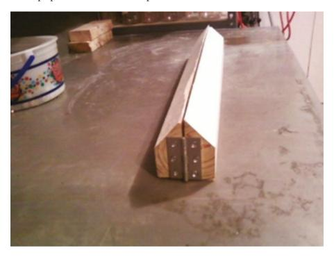
Since I made the boards longer than needed, later I plan on drilling a small hole between the two boards, so that I can insert a vacuum sealer hose inside the bag and can partially evacuate the air before sealing so that I can use a smaller and less expensive  $O_2$  absorber.
