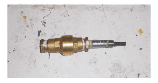
An easy way to measure would be to screw everything together and measure the exposed length of pipe (that way you don't have to keep track of the amount that is threaded). Unscrew everything and rotate the piston to TDC. Insert a rod to measure from TDC to the top of the spark plug hole. The last measurement is from the bottom of the check valve to its open
