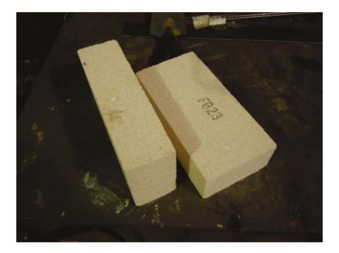
The basis of the forge is a single soft firebrick. I found one at the local ceramic supply store for \$5. Soft firebrick is very light and crumbly—almost like an airy Styrofoam, which is what makes it perfect for this use.
