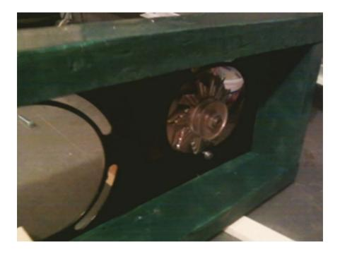
As soon as the paint dried I screwed the plate to the box and attached the alternator. It fits just like an alternator in a car. One screw fits in a whole in the plate, while a bolt fits in an adjustment slot in the plate and through the alternator and locks with a nut. To tighten the belt you loosen the bolt and move the alternator in the adjustment slot.
