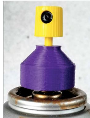
**FIGURE 4.27** – Different angles of the 3D printed adaptor part and nozzle. Jonathan Torta.
