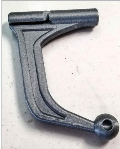
**FIGURE 4.11** – The printed prototype of the HangTime Hook. Jonathan Torta.
