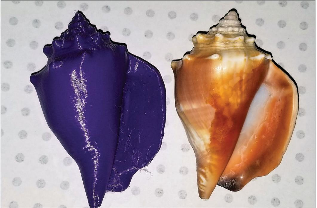
**FIGURE 12.1** - A 3D printed shell and the original. Jonathan Torta.
