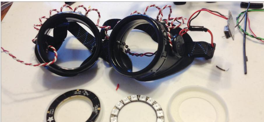
**FIGURE 4.30** – A 3D printed custom ring for inserting and holding the 16 NeoPixel ring in the goggles. Jonathan Torta.
