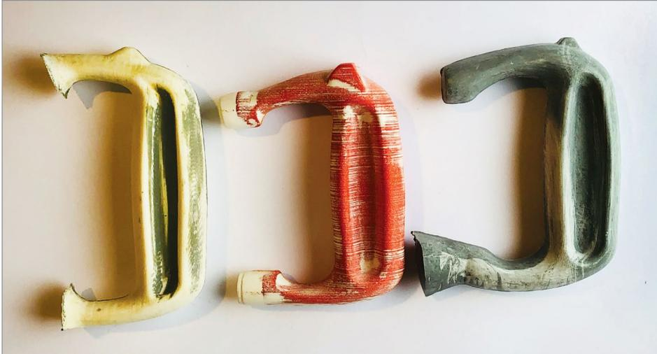
**FIGURE 4.15** – Printing for production A. far left: outsourced 3D printed handle B. middle: 3D printed handle by Jamber using PLA and the Ultimaker 2 C. far right: epoxy handle from 3D print for making master molds. Photo image courtesy of Jamber, Inc.
