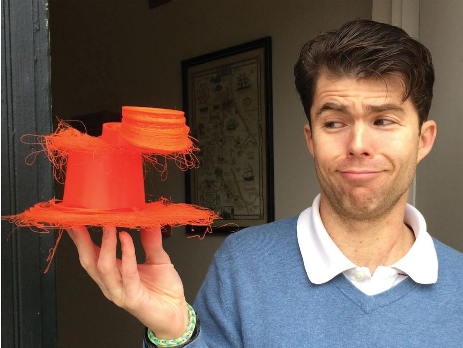
**FIGURE 4.16** – Frustration after finding a 26-hour printing “Beautiful” failure – We came back after 26 hours of printing to find this beautiful mess of a failure. This is just a consequence of printing. We kept some of the cooler failures, such as this beauty. Photo image courtesy of Jamber, Inc.
