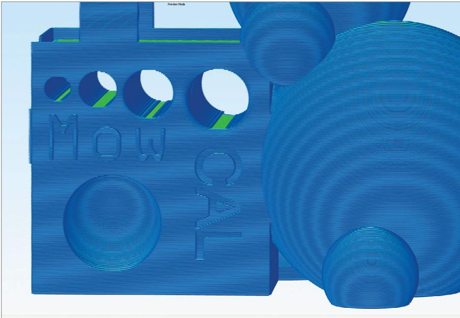
**FIGURE 12.15** – Sliced with words vertically (z-axis) with 0.4 mm nozzle. Jonathan Torta.
