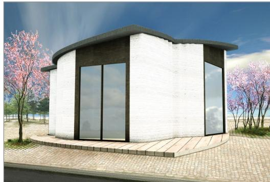
**FIGURE 2.11** – The building-on-demand (BOD) structure is a recently built small office hotel with a 3D-printed wall and foundation structure. This is the first building of its kind in Europe. 3DPrinthuset.
