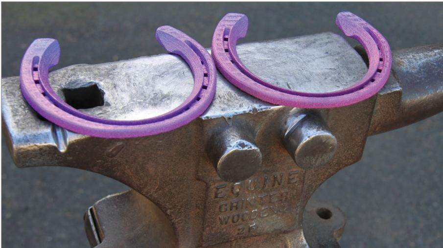
**FIGURE 2.22** – CSIRO scientists have custom made and 3D printed a set of titanium shoes for one Melbourne race horse in a first for the sport. The horse, dubbed by researchers as “Titanium Prints,” had its hooves scanned with a handheld 3D scanner. Using 3D modelling software, the scan was used to design the perfect fitting; lightweight racing shoe and four customized shoes were printed within only a few hours. CSIRO.
